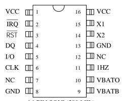
16-PIN SOIC (300 MIL) See Mech. Drawings Section
