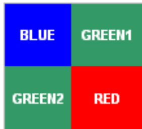
Figure 4. Color Filter Arrangement on the Pixels
