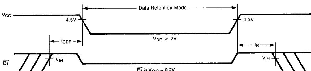
LOW V<sub>CC</sub> DATA RETENTION WAVEFORM (2) (E<sub>2</sub> Controlled)
