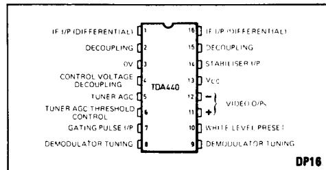
Fig. 1 Pin connections.
