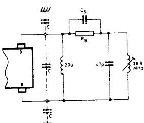
C = Parasitic capacitance at pins 8 and 9 should be kept to a minimum.
