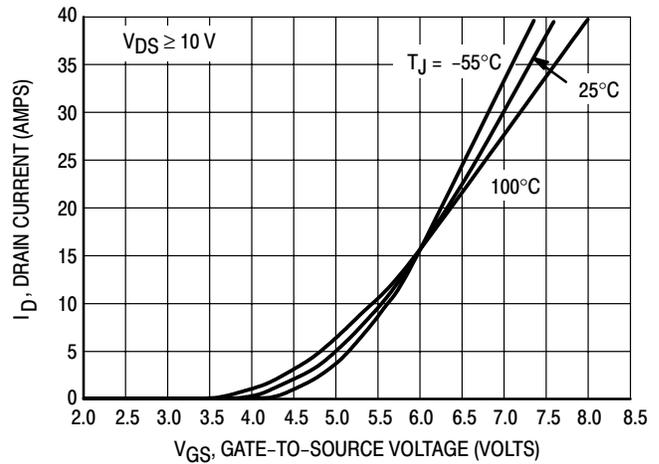
Figure 2. Transfer Characteristics
