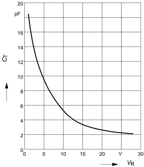
**Normalized diode capacitance**
