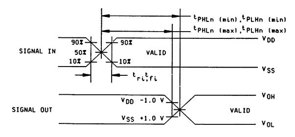
FIGURE 4. Switching test circuit and waveforms - continued.
