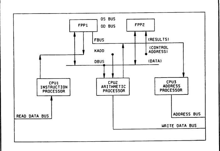
FIGURE 3. Block diagram.
