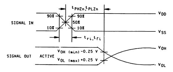
FIGURE 4. Switching test circuit and waveforms - continued.
