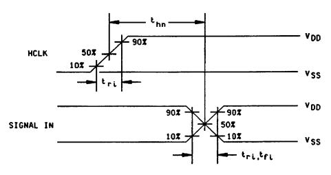
FIGURE 4. Switching test circuit and waveforms - continued.
