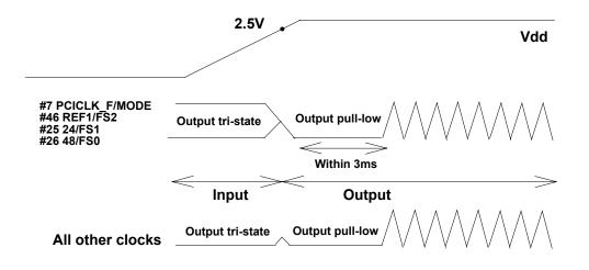
Each of these pins has a large pull-up resistor (250 k $\Omega$  @3.3V) inside. The default state will be logic 1, but the internal pull-up resistor may be too large when long traces or heavy load appear on these
