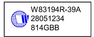
1st line: Winbond logo and the type number: W83194R-39/-39A 2nd line: Tracking code <u>2</u> 8051234 <u>2</u>: wafers manufactured in Winbond FAB 2 <u>8051234</u>: wafer production series lot number 3rd line: Tracking code <u>814 G B B</u> <u>814</u>: packages made in '98, week <u>14</u> <u>G</u>: assembly house ID; A means ASE, S means SPIL, G means GR <u>BB</u>: IC revision
