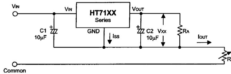
$$I_{OUT} = \frac{V_{XX}}{R_A} + I_{SS}$$
