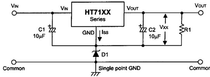
$$V_{OUT} = V_{XX} + V_{D1}$$
