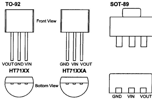
Note: To distinguish the new TO-92 package pin-out (GND VIN VOUT) from the older version (VOUT GND VIN), an HT71XXA mark will be printed on the package while the older version will retain its HT71XX mark.
