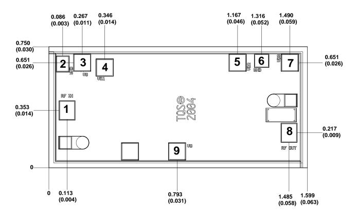
Units: millimeters (inches) Thickness: 0.100 (0.004)
