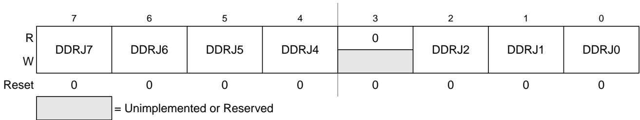
Figure 22-58. Port J Data Direction Register (DDRJ)
