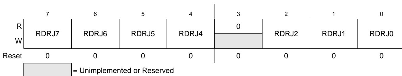
Figure 23-59. Port J Reduced Drive Register (RDRJ)
