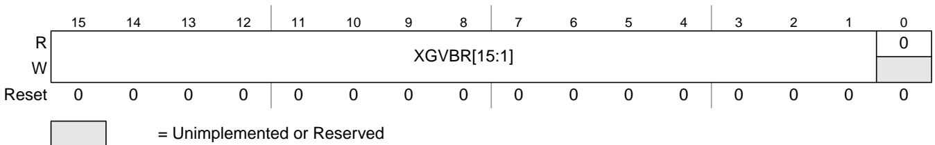
Figure 6-5. XGATE Vector Base Address Register (XGVBR)
