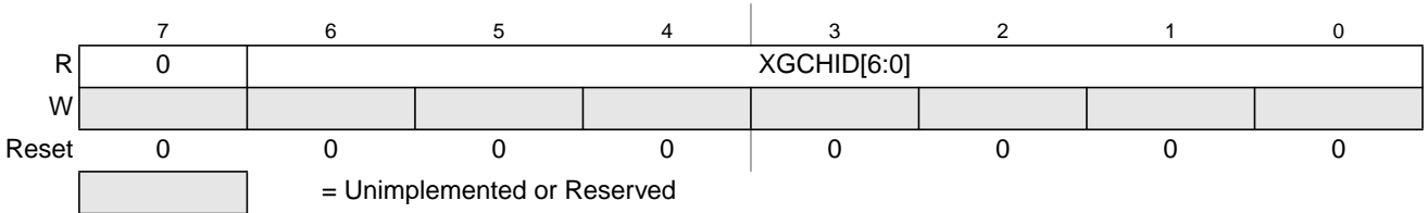
Figure 6-4. XGATE Channel ID Register (XGCHID)
