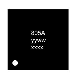
Marking for the 3x3mm MLPD-10 Lead Package: nnnn = Part Number (Example: 805A) yyww = Datecode (Example: 0652) xxxx = Semtech Lot No. (Example: E901)
