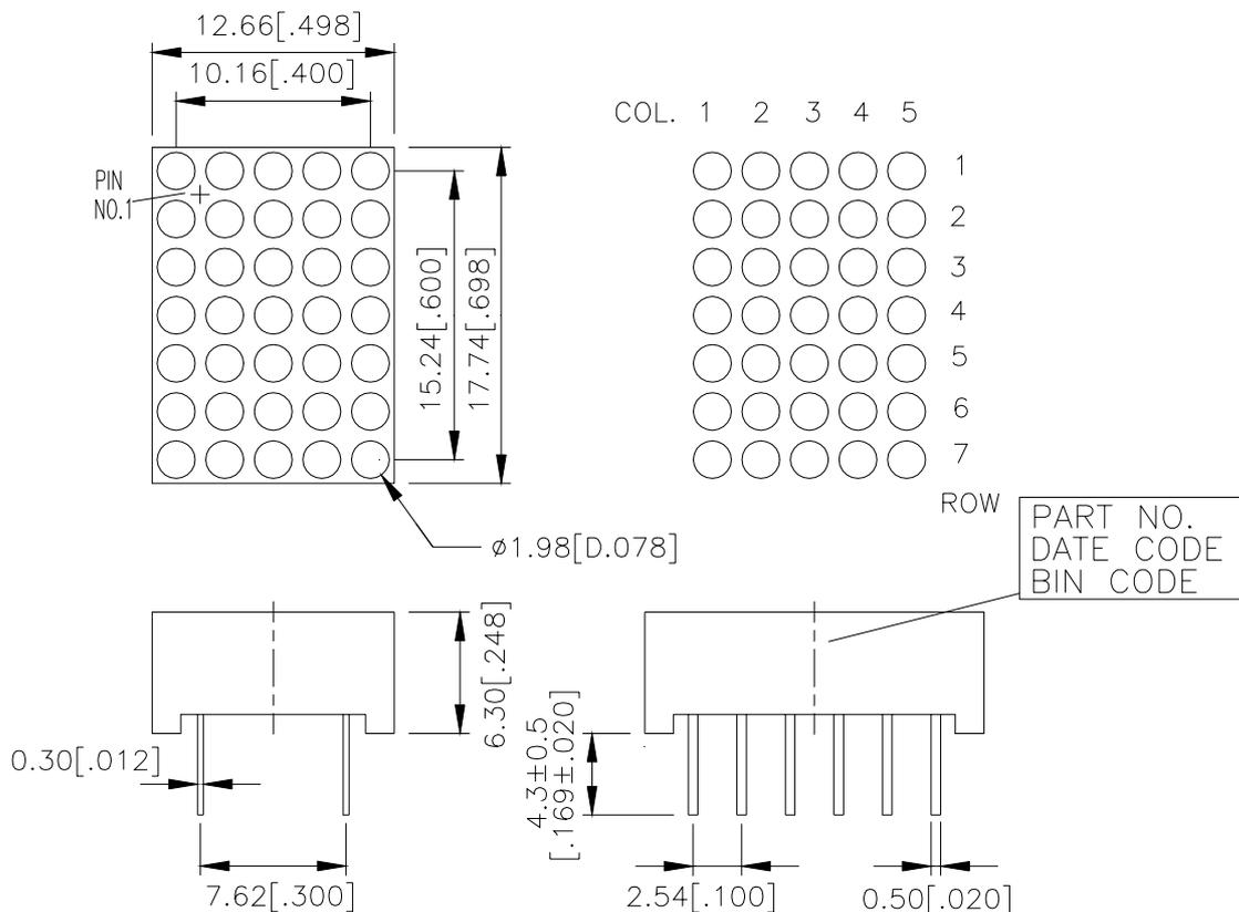
NOTES: All dimensions are in millimeters. Tolerances are  $\pm 0.25$ -mm (0.01<sup>o</sup>) unless otherwise noted.
