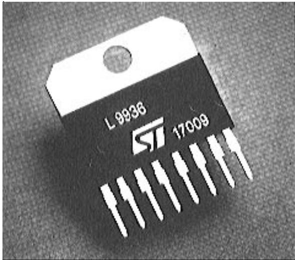
One alternative, widely used in simple power ICs, is to use thick (250 $\mu$ m) aluminum wires. However, a thick aluminum bonding wire needs a large bonding pad on the die. In a simple device like a 3-terminal voltage regulator this is not a problem because there are few such pads, but for more complex ICs with eight or more connections the wasted silicon area would be excessive.
