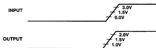
Figure 35. Voltage Reference Levels for AC Measurements (Except Output Enable/Disable)
