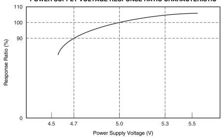
POWER SUPPLY VOLTAGE RESPONSE RATIO CHARACTERISTIC
