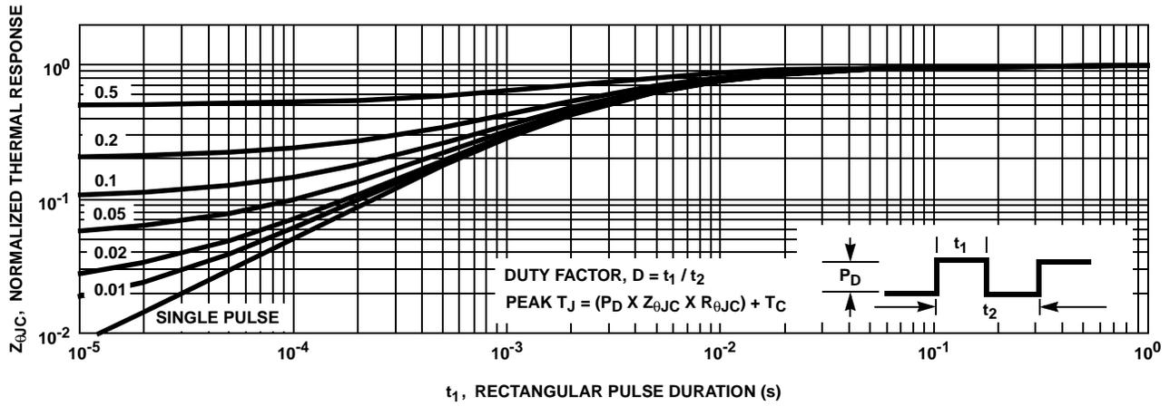
FIGURE 17. NORMALIZED TRANSIENT THERMAL RESPONSE, JUNCTION TO CASE
