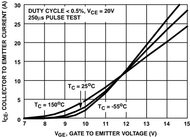
FIGURE 13. TRANSFER CHARACTERISTIC
