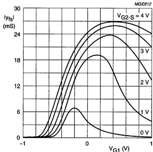
$V_{DS} = 8 \text{ V}; T_{amb} = 25^\circ\text{C}.$
