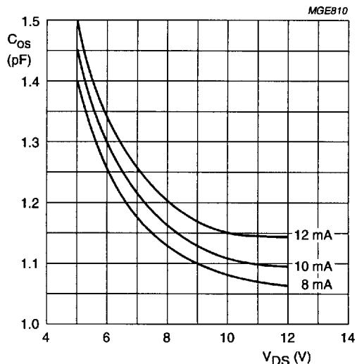
$V_{G2-S} = 4 \text{ V}; f = 1 \text{ MHz}; T_{amb} = 25^\circ\text{C}.$
