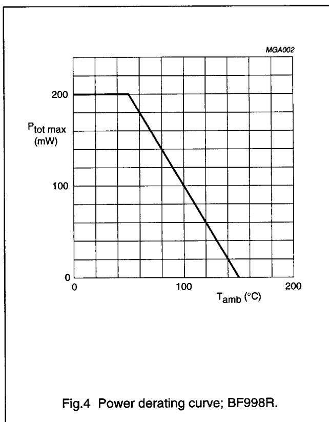
Fig.4 Power derating curve; BF998R.
