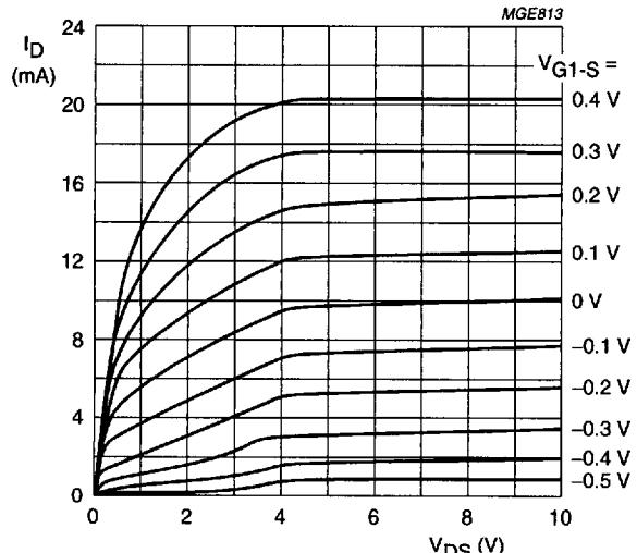
$V_{G2-S} = 4$  V;  $T_{amb} = 25$  °C.
