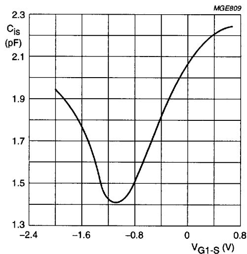
$V_{DS} = 8 \text{ V}; V_{G2-S} = 4 \text{ V}; f = 1 \text{ MHz}; T_{amb} = 25^\circ\text{C}.$
