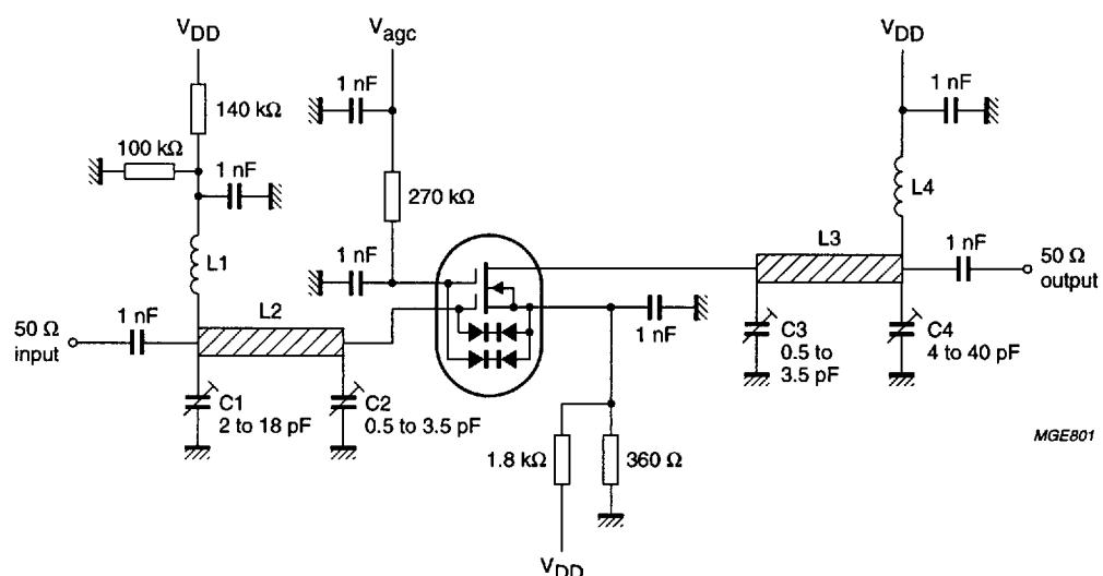
$V_{DD} = 12 \text{ V}$ ;  $G_S = 3.3 \text{ mS}$ ;  $G_L = 1 \text{ mS}$ . $L1 = L4 = 200 \text{ nH}$ ; 11 turns 0.5 mm copper wire, without spacing, internal diameter 3 mm. $L2 = 2 \text{ cm}$ , silvered 0.8 mm copper wire, 4 mm above ground plane. $L3 = 2 \text{ cm}$ , silvered 0.5 mm copper wire, 4 mm above ground plane.Fig.18 Gain control test circuit at  $f = 800 \text{ MHz}$ .
