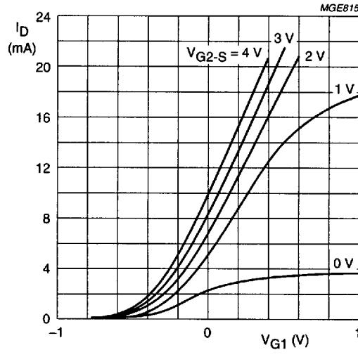
$V_{DS} = 8$  V;  $T_{amb} = 25$  °C.
