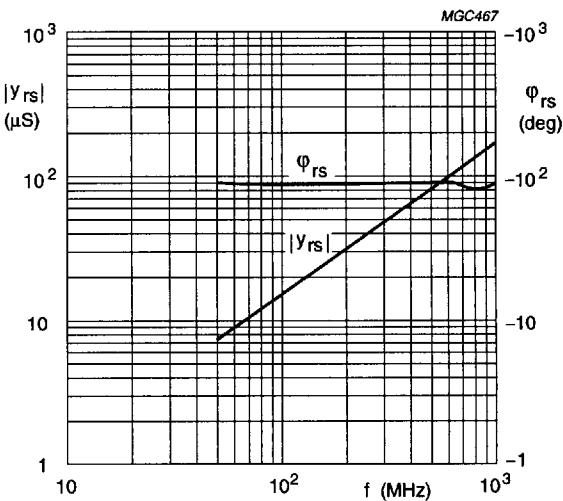
$V_{DS} = 8$  V;  $V_{G2-S} = 4$  V;  $I_D = 10$  mA;  $T_{amb} = 25$  °C.
