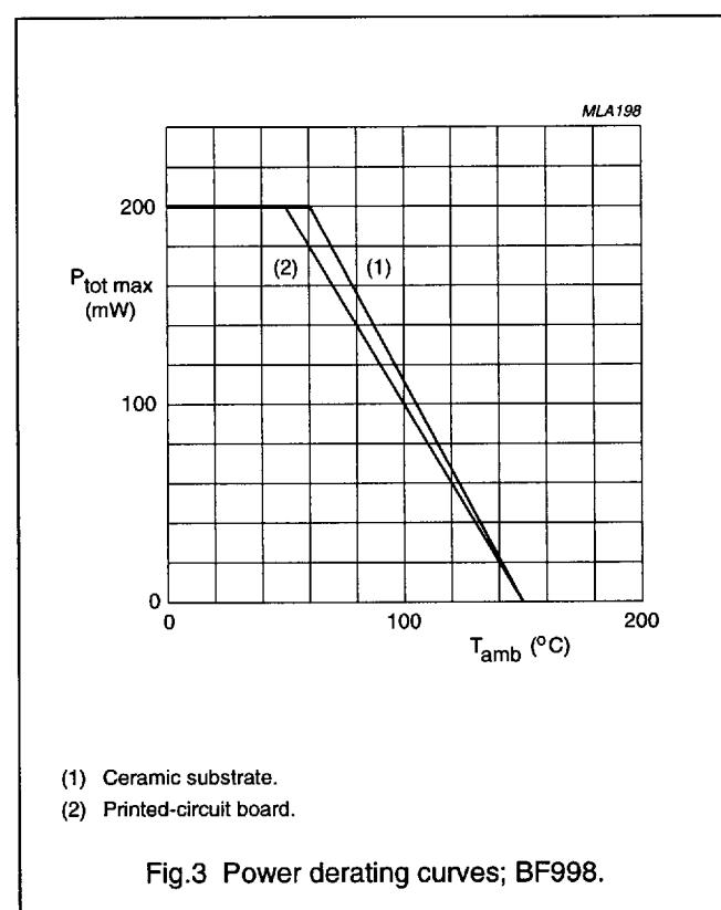
Fig.3 Power derating curves; BF998.
