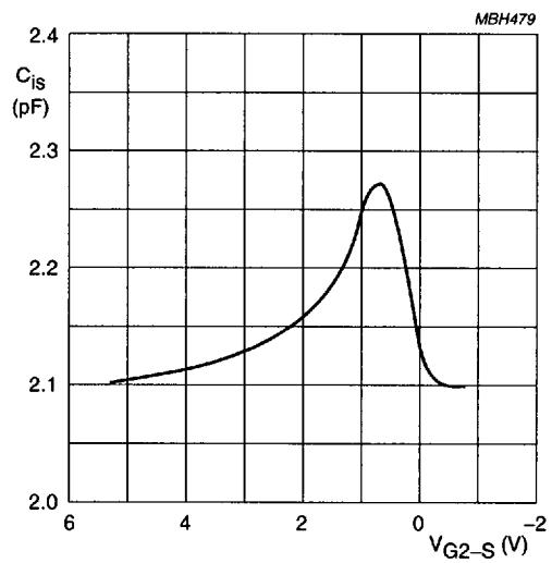
$V_{DS} = 8 \text{ V}; V_{G1-S} = 0 \text{ V}; f = 1 \text{ MHz}; T_{amb} = 25^\circ\text{C}.$
