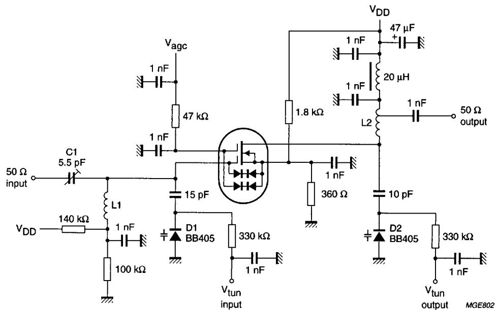
$V_{DD} = 12 \text{ V}$ ;  $G_S = 2 \text{ mS}$ ;  $G_L = 0.5 \text{ mS}$ . $L_1 = 45 \text{ nH}$ ; 4 turns 0.8 mm copper wire, internal diameter 4 mm. $L_2 = 160 \text{ nH}$ ; 3 turns 0.8 mm copper wire, internal diameter 8 mm.Tapped at approximately half a turn from the cold side, to adjust  $G_L = 0.5 \text{ mS}$ .  $C_1$  adjusted for  $G_S = 2 \text{ mS}$ .Fig.17 Gain control test circuit at  $f = 200 \text{ MHz}$ .
