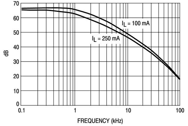
**Figure 13. Ripple Rejection**
