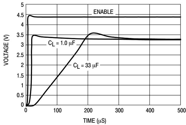
**Figure 14. Enable Transient**
