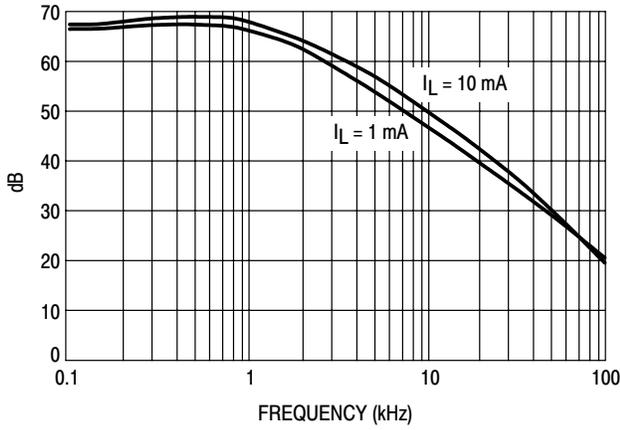
**Figure 12. Ripple Rejection**
