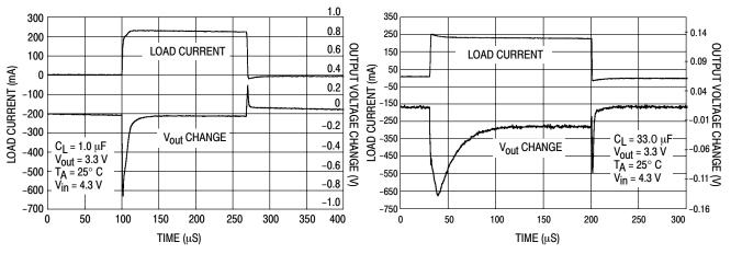
Figure 3. Load Transient Response
