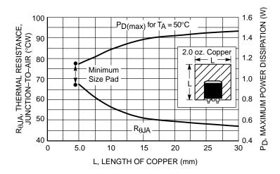
Figure 17. DPAK Thermal Resistance and Maximum Power Dissipation versus P.C.B. Copper Length
