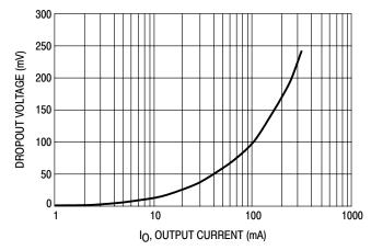
Figure 6. Dropout Voltage versus Output Current
