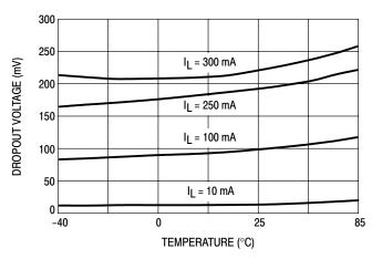
Figure 7. Dropout Voltage versus Temperature
