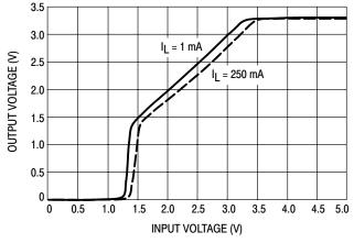
Figure 5. Output Voltage versus Input Voltage
