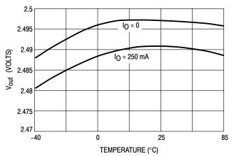
Figure 10. Output Voltage versus Ambient Temperature (V<sub>in</sub> = V<sub>out1</sub> +1V)
