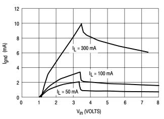
Figure 8. Ground Pin Current versus Input Voltage
