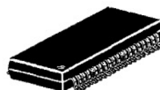
Outline 36P2R-A 0.8mm pitch 450mil SSOP (8.4mmx15.0mmx2.0mm)
