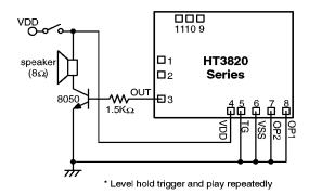
\* Note: The IC substrate should be connected to VDD in the PCB layout artwork.
