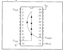
the registered output pins (if they are enabled through  $\overline{OE}$ ) will always be high on power-up, regardless of the programmed polarity of the output pins. This features can greatly simplify state machine design by providing a known state on power-up.
