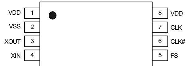
Figure 1. Pin Diagram - 8 Pin TSSOP
