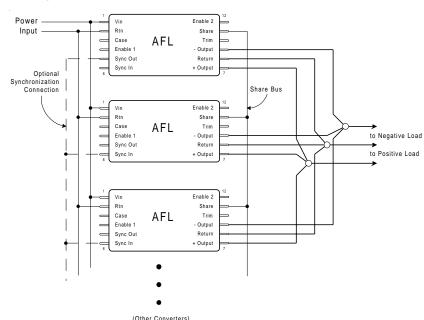
Figure III. Preferred Connection for Parallel Operation
