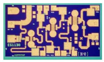
The TriQuint TGA1073A-SCC is a three stage MPA MMIC design using TriQuint's proven 0.25-µm mmW pHEMT 2MI process. The TGA1073A is designed to support a variety of millimeter wave applications including point-to-point digital radio and LMDS/LMCS.
