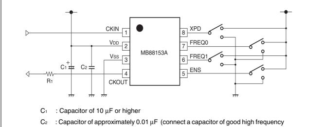
property (ex. laminated ceramic capacitor) to close to this device)
