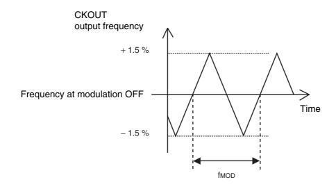
• −1.0% modulation rate, Example of down spread
