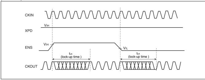
When ENS pin is controlled for enable modulation, it is necessary for the stably clock output from CKOUT pin to wait lock-up time ( $t_{LK}$ ).
