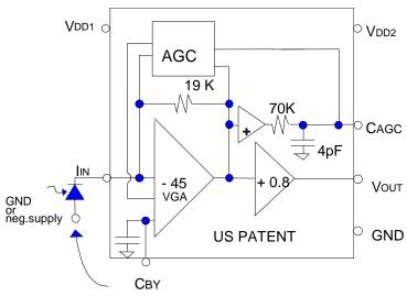
Photodector cathode must be connected to lin for proper AGC operation
