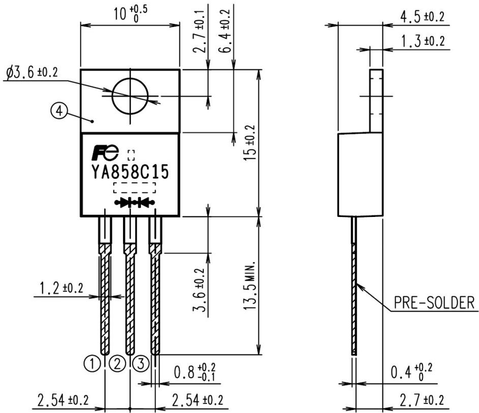
DIMENSIONS ARE IN MILLIMETERS.
