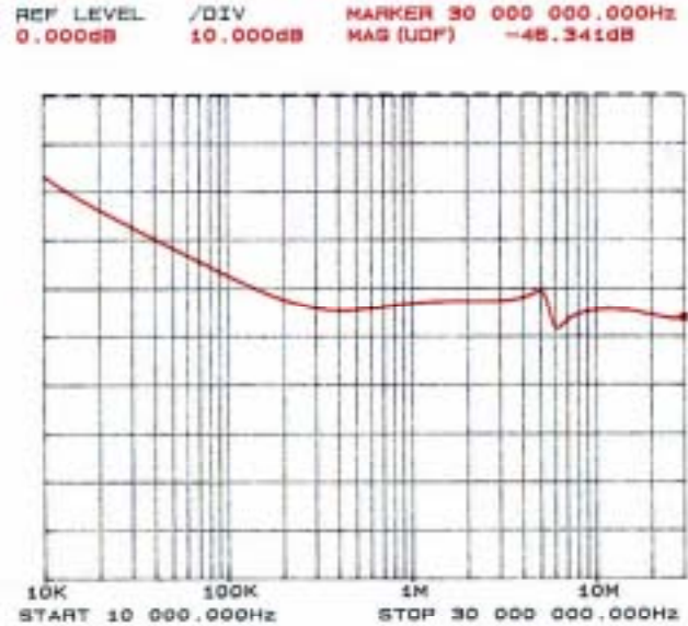
Figure 2: Typical differential-mode insertion loss in a 50 circuit
