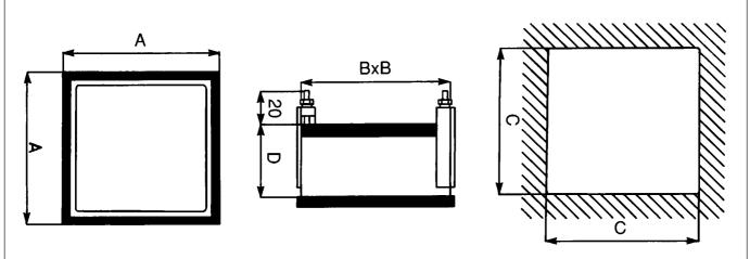
Terminals - M4 Screw Clamps. 48mm Voltmeters - 6.3 x 0.8 Push-on Tags
