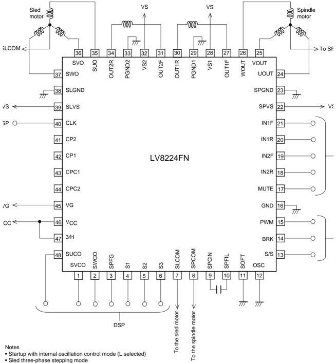
Cored motor spindle motor mode
