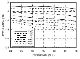
Attenuation vs. Vcnrl1 Over Temperature @ 30 GHz, Vctrl2 = -3V
