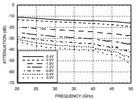
Attenuation vs. Vcntrl2 Over Temperature @ 30 GHz, Vctrl1 = 0V
