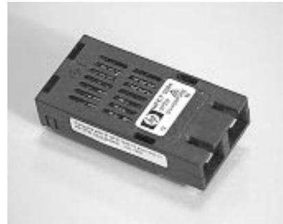
The new multisourced 2 x 9 footprint package style is a variation of the standard 1 x 9 package with an integral Duplex SC connector receptacle. The extra row of 9 pins provides connections for laser bias and optical power monitoring as well as providing transmitter disable function. A block diagram is shown in Figure 1.
