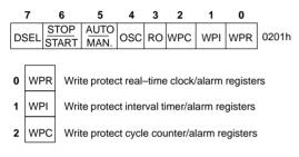
Setting a write protect bit to a logic 1 will permanently write protect the corresponding counter and alarm registers, all write protect bits, and additional bits in the control register. The write protect bits can not be written in a normal manner (see "Write Protect/Programmable Expiration" section).
