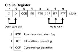
When a given alarm occurs, the corresponding alarm flag is set to a logic 1. The alarm flag(s) is cleared by reading the status register.
