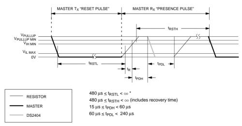
\*In order not to mask interrupt signaling by other devices on the 1–Wire bus, t<sub>RSTL</sub> + t<sub>R</sub> should always be less than 960 µs.
