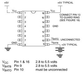
To always allow communication through the 1–Wire or 3–wire port, the voltage on  $V_{CC}$  must be approximately
