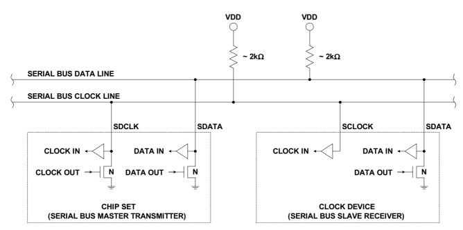
Figure 1. Serial Interface Bus Electrical Characteristics
