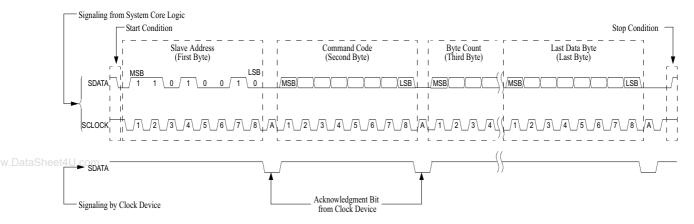
Figure 4. Serial Data Bus Write Sequence
