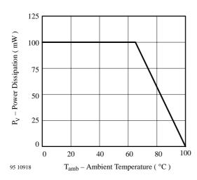
Figure 1. Power Dissipation vs. Ambient Temperature
