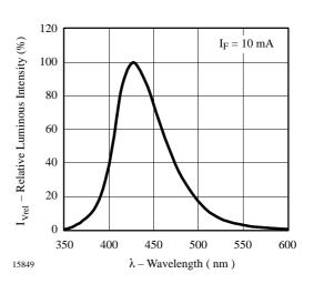
Figure 7. Relative Luminous Intensity vs. Wavelength
