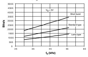
Figure 6-7. Typical Bandpass Curve
