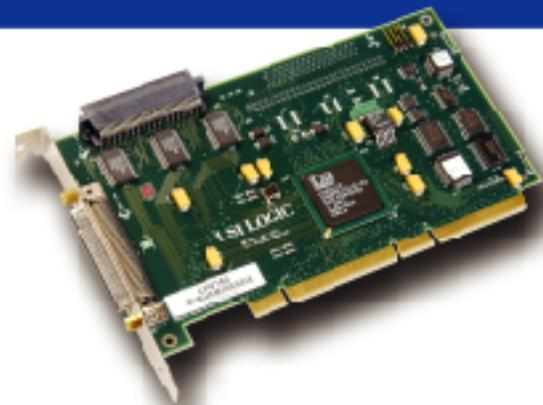
*The LSIU160 Ultra160 SCSI host adapter is the best solution to connect to high performance Ultra160 hard disks drives.*
