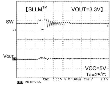
Fig. 14 SW waveform I<sub>o</sub>=10mA
