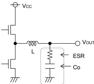
Fig.28 Output capacitor
