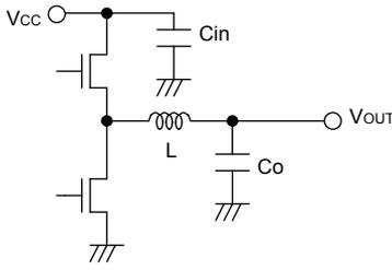
Fig.29 Input capacitor
