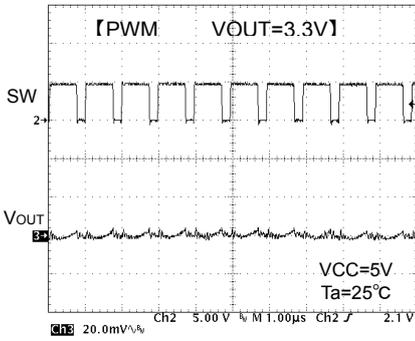
Fig. 15 SW waveform I<sub>o</sub>=3A
