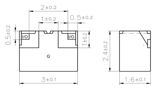
View from below onto the solder terminals and view from beside Marking: 'EPCOS logo', on top of the filter
