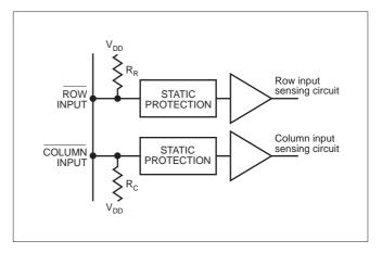
Figure 6: Row and Column inputs
