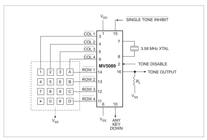
Figure 7: Connection diagram
