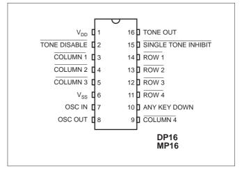
Figure 1: Pin connections - top view
