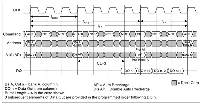
Figure 14 Single READ Burst (CAS Latency = 3)
