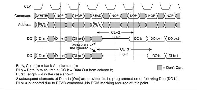
Figure 33 WRITE to READ Timing
