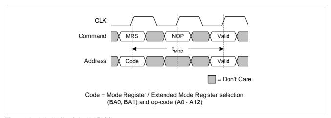
Figure 8 Mode Register Definition
