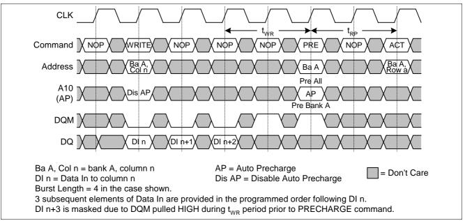
Figure 34 WRITE to PRECHARGE Timing
