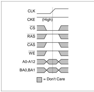
The NO OPERATION (NOP) command is used to perform a NOP to a Mobile-RAM which is selected ( $\overline{CS}$  = LOW). This prevents unwanted commands from being registered during idle states. Operations already in progress are not affected.
