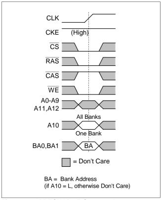
The PRECHARGE command is used to deactivate (close) the open row in a particular bank or the open row in all banks. The bank(s) will be available for a subsequent row access a specified time ( $t_{\rm RP}$ ) after the PRECHARGE command is issued. Input A10 determines whether one or all banks are to be precharged, and in the case where only one bank is to be precharged, inputs BA0, BA1 select the bank. Otherwise BA0, BA1 are treated as "Don't Care".
