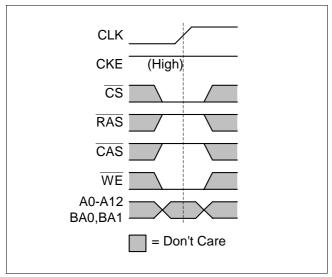
Figure 35 BURST TERMINATE Command
