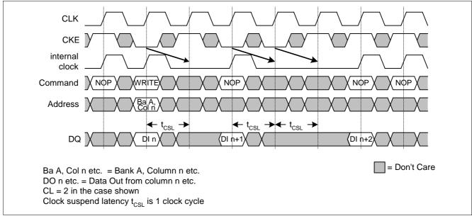
Figure 31 Clock Suspend Mode for WRITE Bursts
