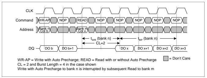
Figure 39 WRITE with Auto Precharge Interrupted by READ
