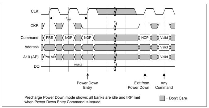
Figure 46 Power Down Entry and Exit
