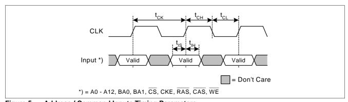
Figure 5 Address / Command Inputs Timing Parameters
