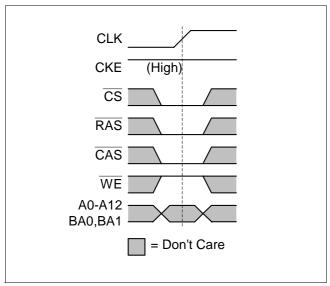
Auto Refresh is used during normal operation of the Mobile-RAM. The command is nonpersistent, so it must be issued each time a refresh is required. A minimum row cycle time ( $t_{\rm RC}$ ) is required between two AUTO REFRESH commands. The same rule applies to any access command after the auto refresh operation. All banks must be precharged prior to the AUTO REFRESH command.
