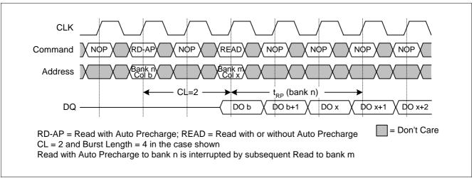
Figure 37 READ with Auto Precharge Interrupted by READ
