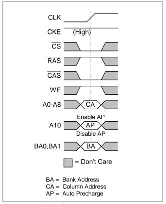
Subsequent to programming the mode register with CAS latency and burst length, READ bursts are initiated with a READ command, as shown in Figure 11. Basic timings for the DQs are shown in Figure 12; they apply to all read operations and therefore are omitted from all subsequent timing diagrams.
