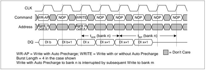
Figure 40 WRITE with Auto Precharge Interrupted by WRITE
