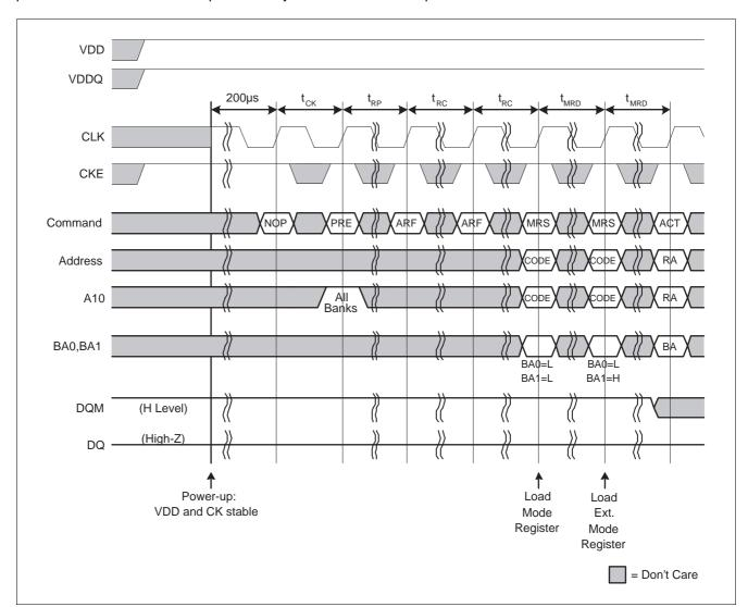
Figure 3 Power-Up Sequence and Mode Register Sets
