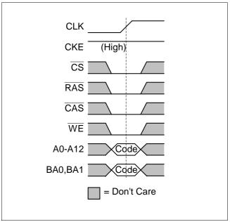
The Mode Register and Extended Mode Register are loaded via inputs A0 - A12 (see mode register descriptions in Chapter 2.2). The MODE REGISTER SET command can only be issued when all banks are idle and no bursts are in progress. A subsequent executable command cannot be issued until  $t_{\rm MRD}$  is met.
