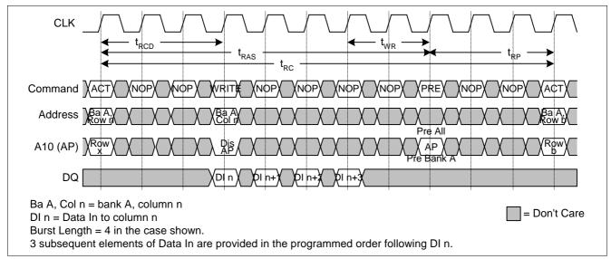
Figure 26 WRITE Burst (CAS Latency = 3)
