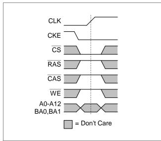
Figure 45 Power Down Entry Command
