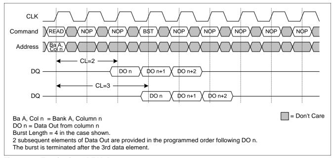
Figure 18 Terminating a READ Burst
