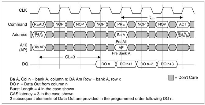
Figure 22 READ to PRECHARGE Timing
