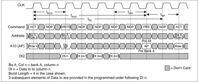
Figure 25 WRITE Burst (CAS Latency = 2)
