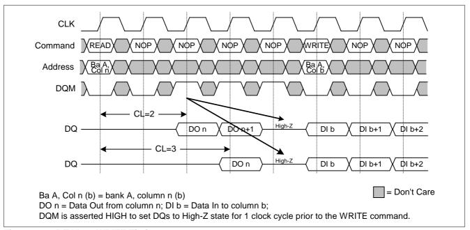
Figure 21 READ to WRITE Timing
