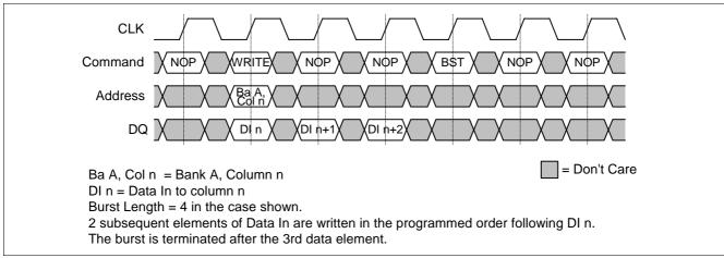
Figure 30 Terminating a WRITE Burst
