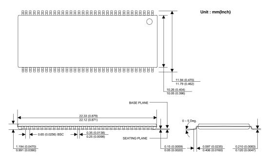
Note: Package do not mold protrusion. Allowable protrusion of both sides is 0.4mm.
