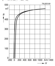
DC magnetic bias measured on ETD cores  $(\hat{B} \le 0.25 \text{ mT}, f = 10 \text{ kHz}, T = 25 ^{\circ}\text{C})$
