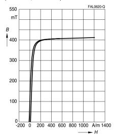
DC magnetic bias measured on ETD cores  $(\hat{B} \le 0.25 \text{ mT}, f = 10 \text{ kHz}, T = 100 ^{\circ}\text{C})$
