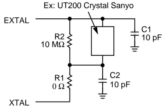
Note: R1 can be increased in size to be used as a current limiter, if needed.
