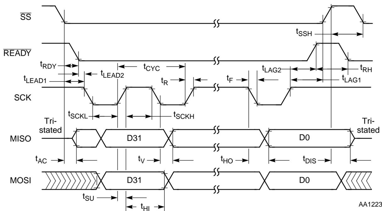
Figure 2-3 SPI Timing
