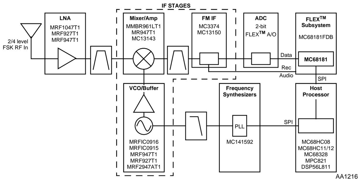
**Figure 4-1** Roaming FLEX™ chip System Block Diagram
