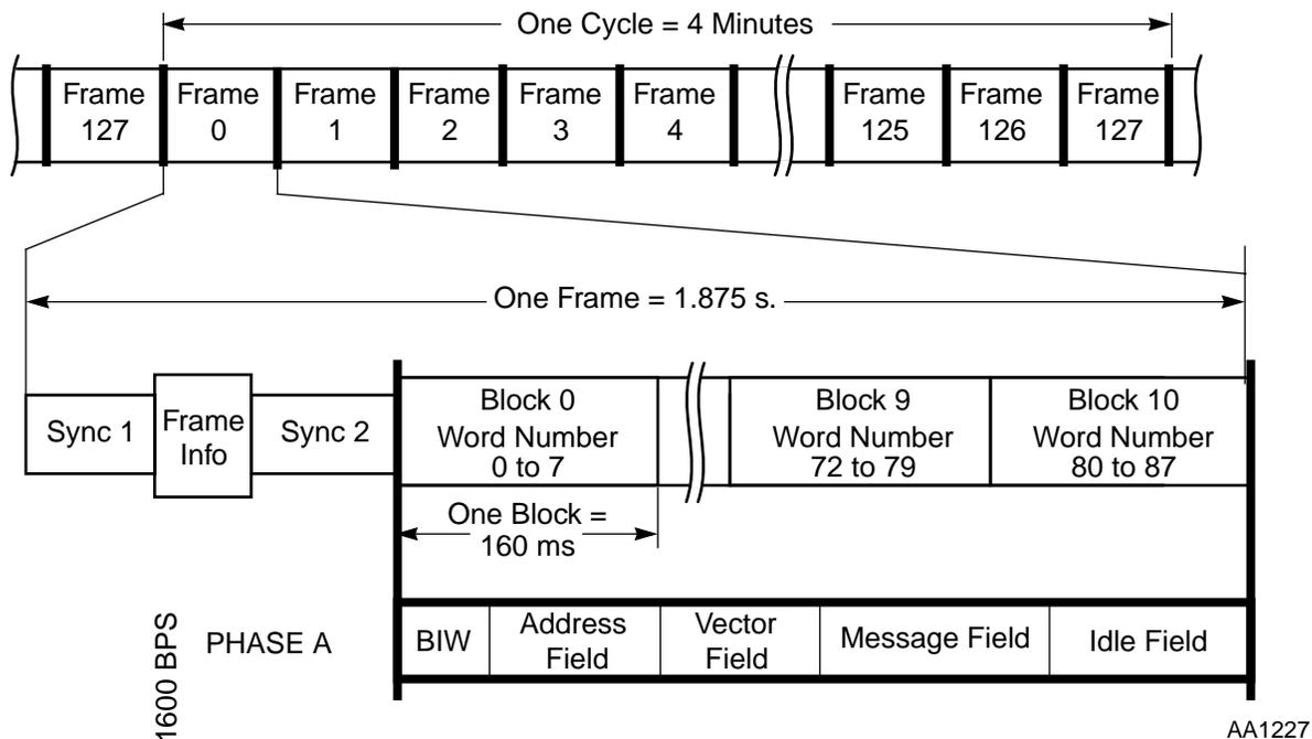
**Figure A-2** FLEX™ Signal Structure for 1600 BPS
