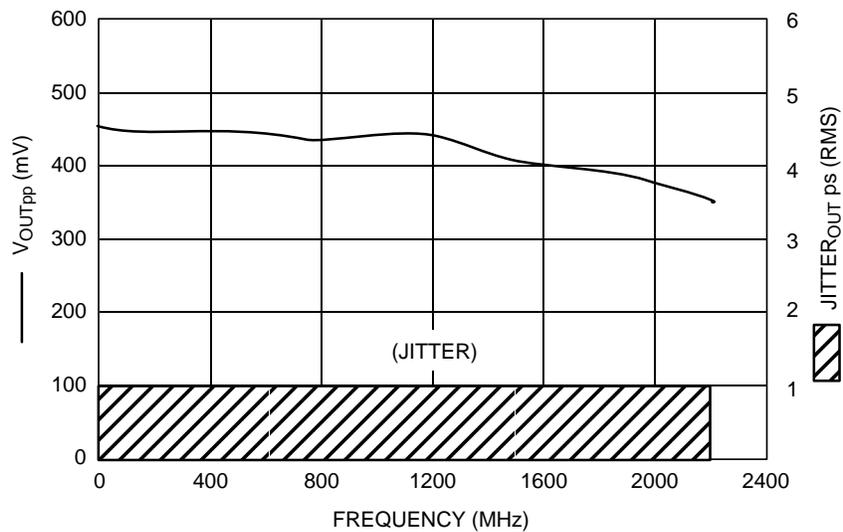
Figure 4.  $F_{\text{max}}/\text{Jitter}$
