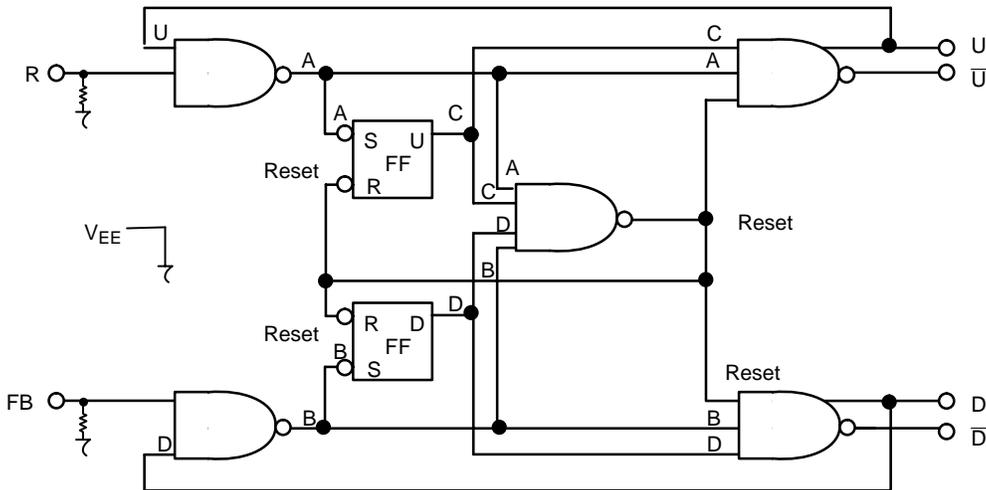
Figure 3. Logic Diagram
