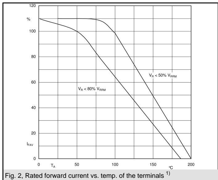
Fig. 2, Rated forward current vs. temp. of the terminals<sup>1)</sup>
