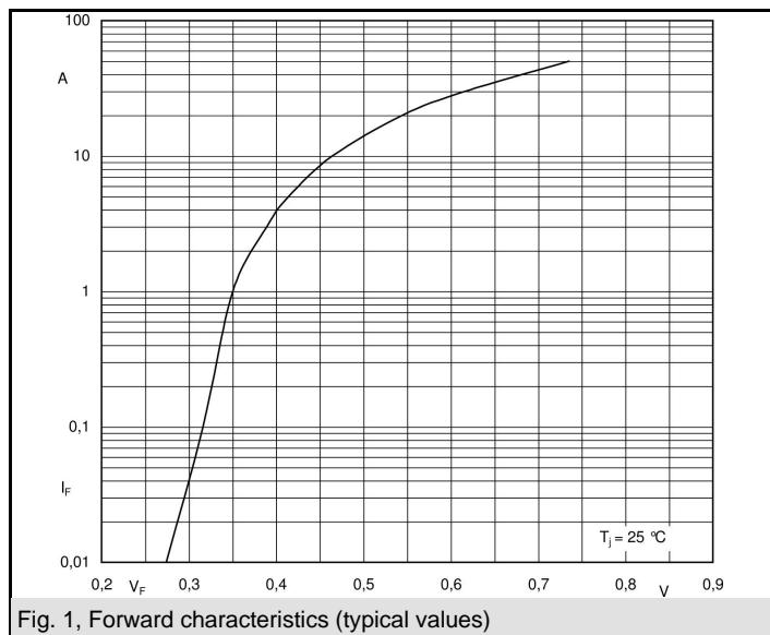
Fig. 1, Forward characteristics (typical values)
