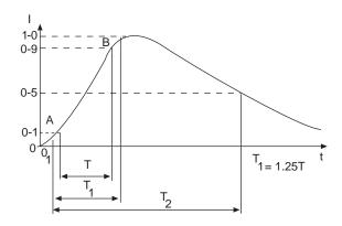
**Maximum Discharge Current** - defined as the peak current of an impulse which the device can withstand once without substantially affecting device performance.
