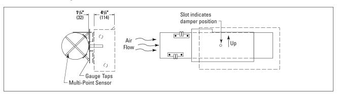
www.Deamperfortation is always clockwise to the open position. An identification mark on the end of the shaft indicates the damper position. Capped "T"s are provided in the sensing lines from the amplifying sensor. These allow field connection of a differential pressure gauge for accurate air flow measurement.
